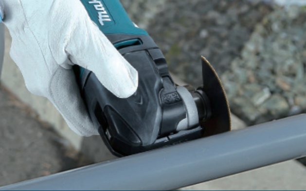
Cutting PVC, FRP pipes
